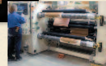
Multek slitting machine for flexible printed circuits
