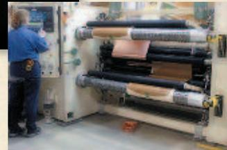
Multek slitting machine for flexible printed circuits
